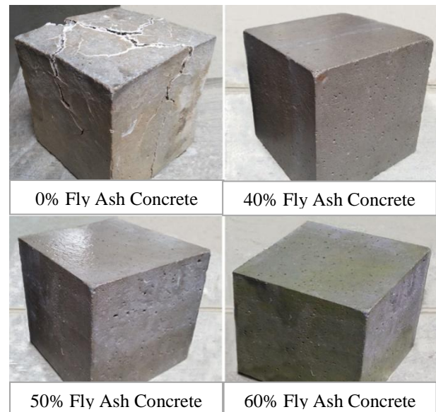
Fig -6: Concrete Specimen after Exposure to Sulphate Solution for 550 days
