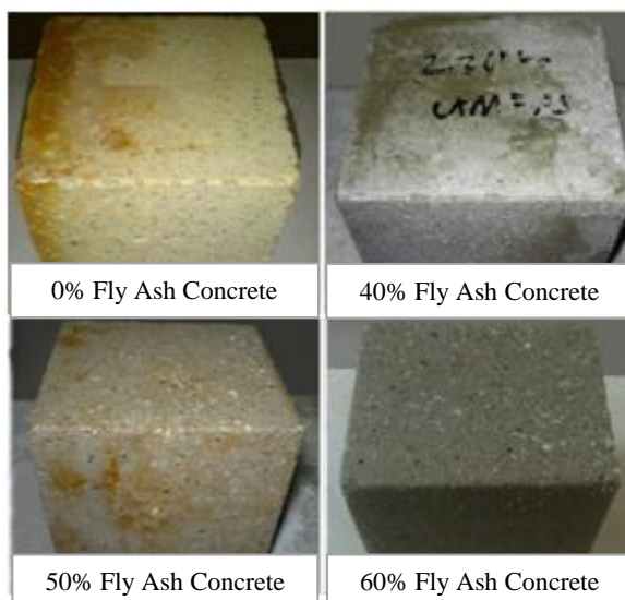
Fig -5: Concrete Specimen after Exposure to Acid for 1800 Hours
