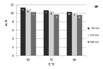
Fig. 1 – Effect of drying air temperature and duration of fluid-bed drying on moisture content (w) of grape pomace (statistically significant difference is marked with different Latin letters, p < 0.05)
