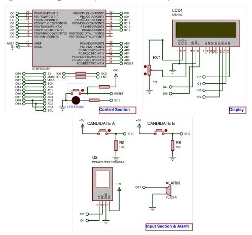
Figure 1 Circuit diagram of EVM (see online version for colours)
