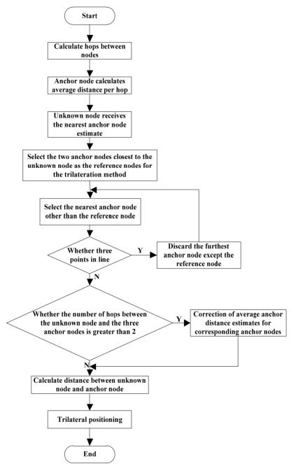
After the initialisation of wireless sensor network, the number of hops between nodes is calculated, in which the anchor node calculates the average per hop distance, while the unknown node receives the closest estimate of the anchor node distance. The two anchor nodes closest to the unknown node are selected as the reference node of trilateral
