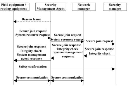
TCC strategy mainly uses the key management tree to manage the network key. The key types in the network can be divided into temporary shared key, personal key, pair key, cluster key, group key and communication key.
