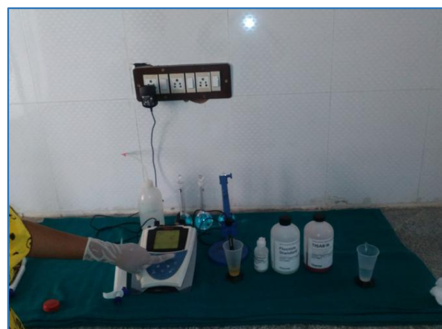
Figure 4. Instrument in use for Measuring Water Fluoride Level
