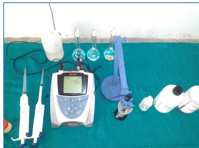
Figure 3. Instrument for Measuring Water Fluoride Level
