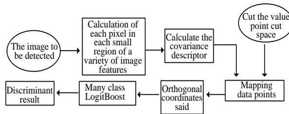
**Figure 2. Flow Chart of Head Poses Recognition**
