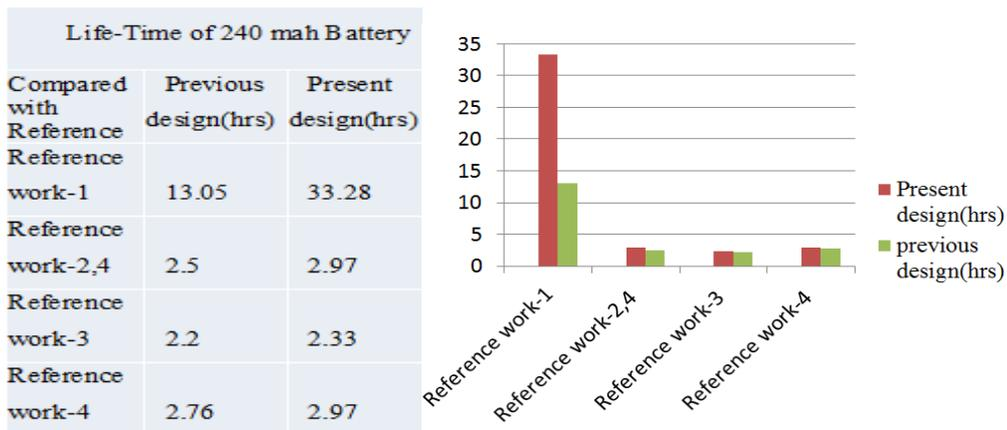
**Figure 8. Life-time of Lithium Coin 240 mah Battery**
