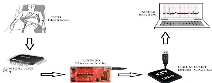
Figure 2. Flow Diagram of ECG System Design
