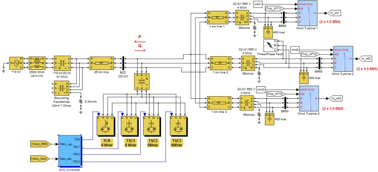
**Fig. 4.** Matlab-Simulink simulation of a wind power station connected to the grid
