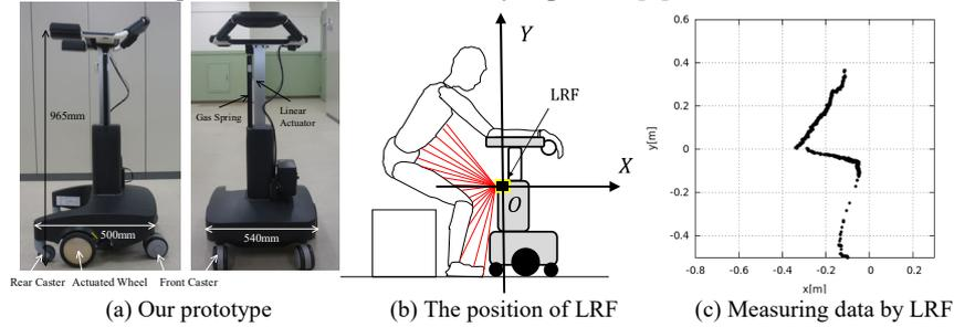
Figure 4. Our prototype and an equipped 2D laser range finder.
