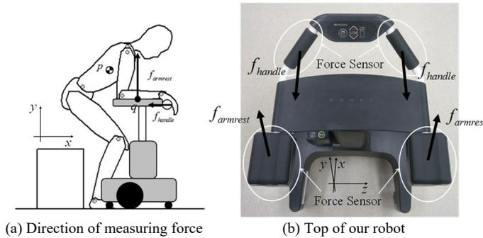
Figure 7. Force sensors equipped on our robot
