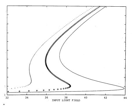
Fig. 2. The output light field  $E_{out}$  versus the input light field  $E_{int}$  with C = 30,  $\xi_1 = \xi_2 = 0$ ,  $\delta = 0$  and  $\rho = 0$  (solid curve);  $\rho = 0.3$  (curve with squares) and  $\rho = 0.6$  (curve with dots).
