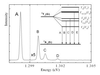
Fig. 1. Representative luminescence spectrum of bulk GaN:Fe crystal measured at 4.2 K. The inset shows the scheme of possible transitions between  ${}^{4}T_{1}(G)$  and  ${}^{6}A_{1}(S)$  states of Fe<sup>3+</sup> ion in GaN (after Ref. [5]).
