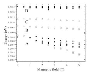
Fig. 4. Energy dependence of all the sublevels of the  ${}^{4}T_{1}(G)$  multiplet on magnetic field up to 5 T, obtained on the basis of photoluminescence data, as described in the text. Let us note the energy scale brake and its magnification below 1.3 eV.
