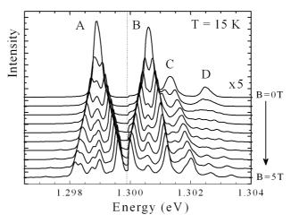
Fig. 3. Luminescence spectra of GaN:Fe measured at 15 K and at magnetic field up to 5 T, applied along *c*-axis.
